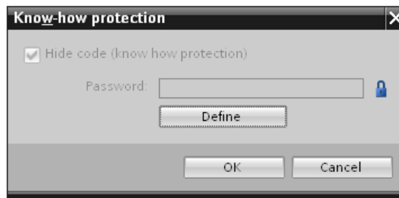
Figure 9-3 Setting up block know-how protection (2)
