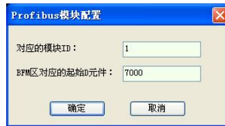
Figure 2-14 Profibus module configuration
