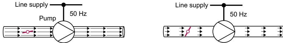
Figure 6-95 Flow control with pump and throttle connected to a 50 Hz line supply
