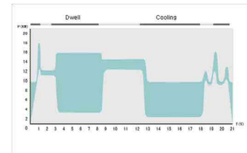
Servo Hydraulic system energy-saving rate is determined by Dwell & Cooling time in the molding cycle.
