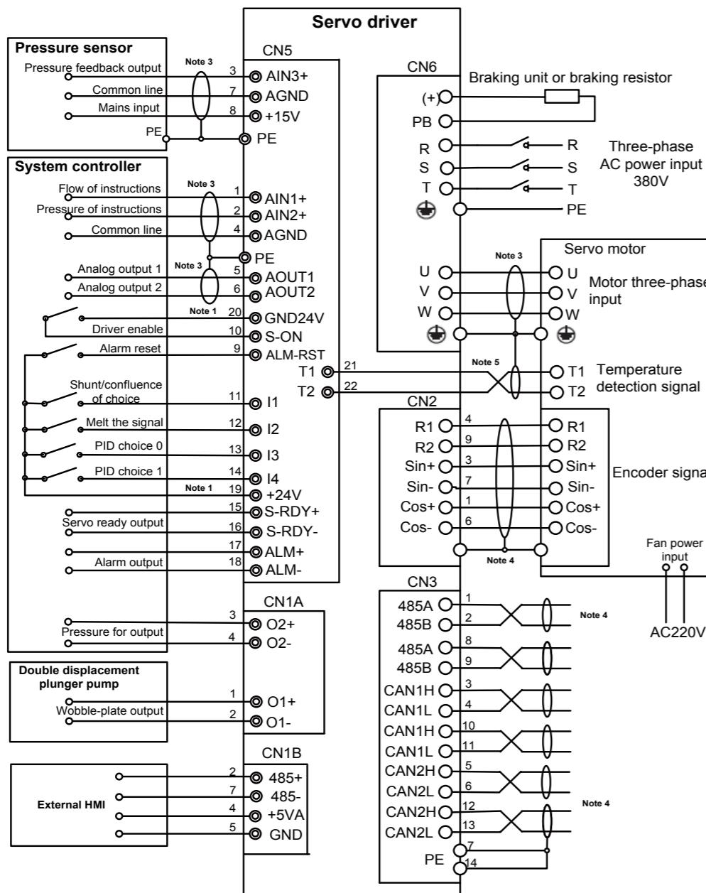
Note 1: in the wiring diagram, the digital input signal using the system controller power to drive, CN5 connector' 24V power from the external. The power of the pressure sensor can also be used drive internal power supply. By jumper J1 to 15 v, connect the + 15 v and + 24 v, through the jumper J2 to 15 v, connect the AGND and GND24V. Drives the factory default J1 and J2 jumper to 15 v side, using drive pressure sensor power supply.
